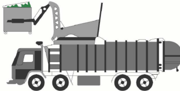
Front-lift-loading waste collection vehicle
